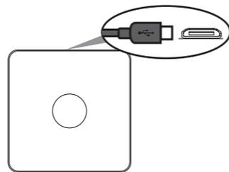
1. Plug one end of the provided micro USB cable into the Wireless Charging pad. Plug the other end into a USB charger or other USB power source.
